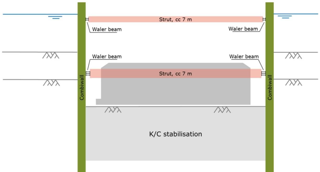
Figure 4. Principle of the open construction pit alternative
