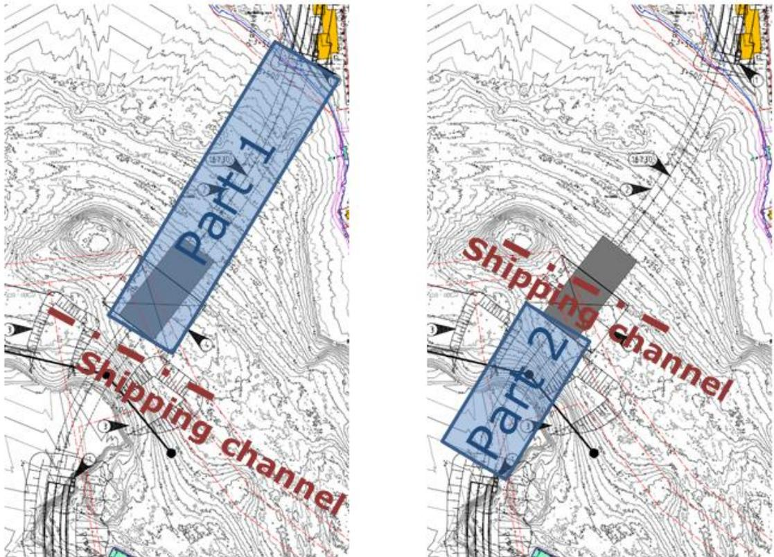
Figure 5. First and second part of the overall construction sequence, that allows the shipping channel to be kept open during construction.
