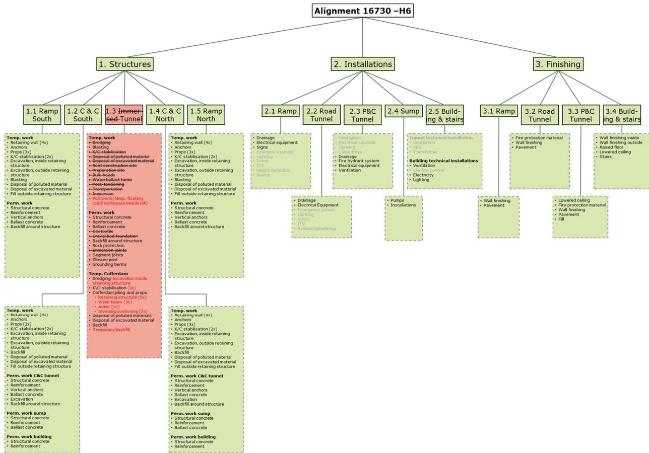
Figure 7. WBS for the open construction pit alternative for tunnel.
